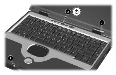
Identifying the power/standby light, power button, and display switch
